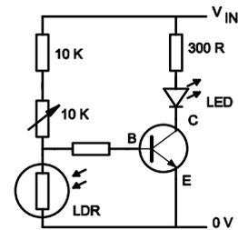
LDR – Light sensor suitable for circuit
