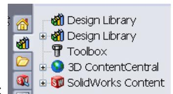
**Note:** Click **Tools, Add-Ins., SolidWorks Toolbox** and **SolidWorks Toolbox Browser** to activate the SolidWorks Toolbox.
