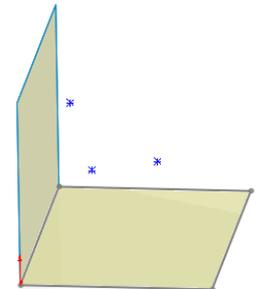
Using the **Point** command from the **Sketch** toolbar, drop **3** points into the sketch as shown. Select **OK** ✓ and press escape to exit the **Point** command.
