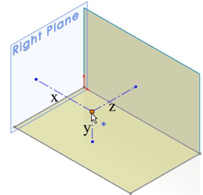
Using the **front view** we can see the **X** and **Y** values; using **top view** we can see the **X** and **Z** values; use the **right view** to see the **Y** and **Z** values.
