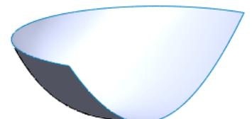
To give the spoon wall a thickness we use the **Thicken** command
