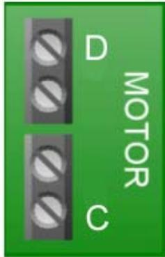
There are two main methods of controlling motors. One method uses the L293D and we also use a double set of relays. Note however that the L293D can only carry around 600mA of current and many motors have a much higher requirement than this. One of the ICs on the board is an L293D and we can connect two motors into positions C and D.
