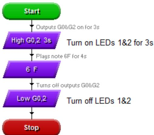
It is possible to turn on a number of outputs at the same time by setting the correct 'bits'. Each bit controls one output. In this case two LEDs are driven from output G0 and output G2.
