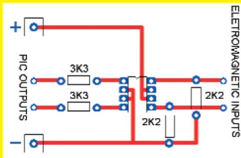
The outputs from the opto-isolator can then be connected to a power transistor such as the BC639.
