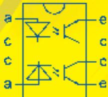
Inside this chip there are two opto-isolators. As can be seen there are two diodes that emit infra red light when current flows through them. There are two transistors whose bases are infrared light sensitive. When infrared light falls onto the base the transistors conduct, when no infrared light is present the transistors are insulators.
