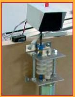
This model camera shows a typical layout using a bent aluminium strip to activate the limit switches and a Universal Gearbox with extra gears. The programmes were varied with some wanting pauses at certain points, but a basic programme did nothing until a switch was turned on and then the camera moved in one direction and the LED flashed until it hit the limit switch and the camera reversed direction until it hit the other limit switch.
