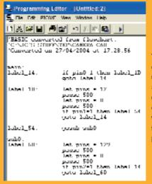
The programme can then be easily modified or improved until the desired outcome is achieved. The ease with which changes can be made and downloaded to the chip, without the need for removing the PIC from the pupils circuit is a major plus for PICAXE.
