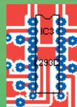
There are a couple of small points worth mentioning, pin 8 and 9 of the motor driver chip are coupled together with a wire link to provide the same battery supply to each motor using the pads below the pins. The pad joined to the left of pin 8 allows for a separate power supply positive connection and the pad directly below the 0v connection.
