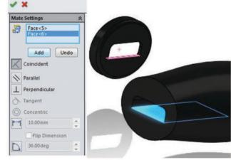
Select the front face of the handle and the back of the washer, and select **Add** to complete this mate also.
