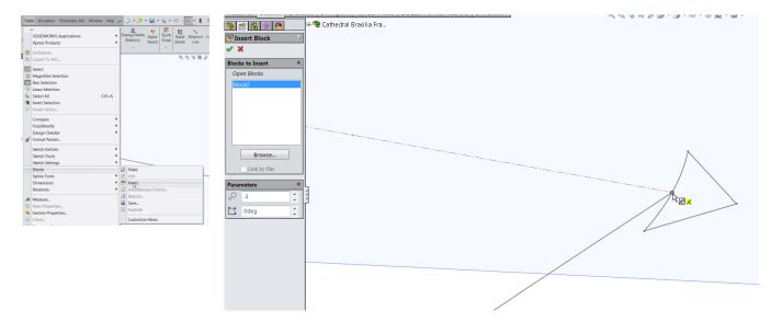
Repeat the block command using the same method and details on  $\bf Plane\ 3$  on the top of the hyperbolic path
