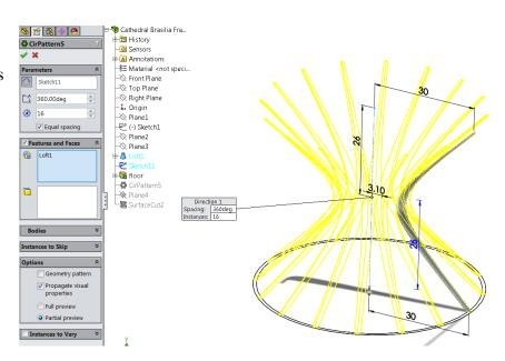
Insert a plane **40m** above the Top Plane. Use the **Cut with surface** command to remove the top of the structure with this surface plane
