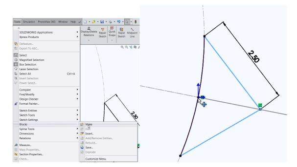
Create a sketch on the **Top Plane.** Insert the block, changing the scale to **0.5** and coincident with the end of the hyperbolic sketch.
